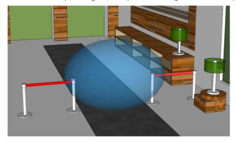
• SNOOPER-DP system forms the **OVAL-SHAPED** (blue area in the picture) detection space between two sensors and can detect the iron objects those are passing between two SNOOPER sensor.
